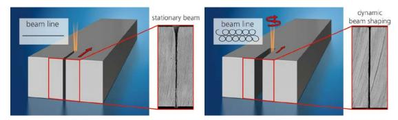
Manipulation of the cut kerf geometry depending on the oscillation function; on the left: conventional cutting process on the right: improved parallelism of the cut kerf by dynamic beam oscillation functions © Fraunhofer IWS Dresden
